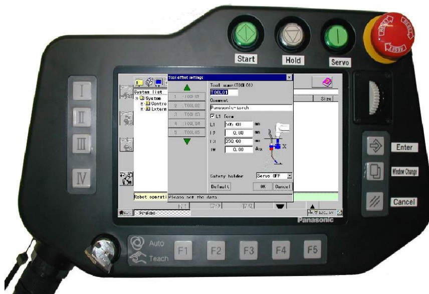
Fig. 2.51 – Teaching Box usado nos robôs da Panasonic.
